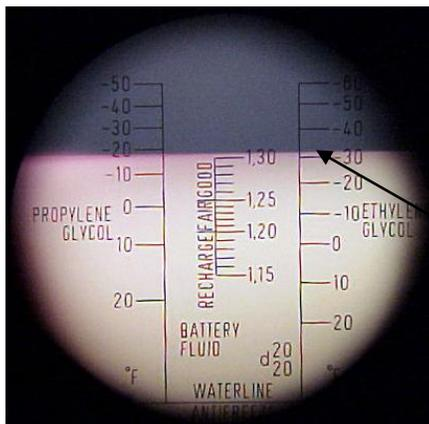
Where the shadow crosses the scale is the correct freeze point reading.
