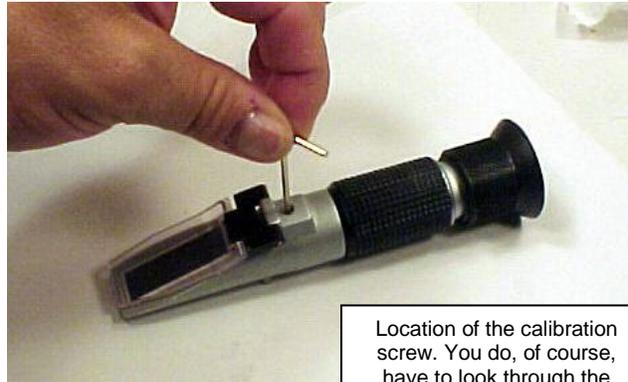
Location of the calibration screw. You do, of course, have to look through the eyepiece while adjusting the calibration!
